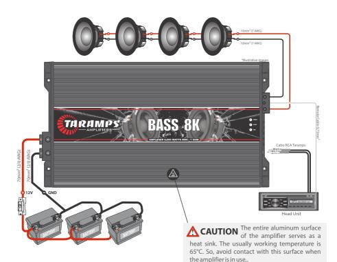
Examples of connections in the power supply input. Note: Required battery bank capacity: At least 320Ah
