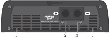
**1 - FANS:** This amplifier has two internal ventilation fans. For perfect functioning, the amplifier must be installed in a cool and aired place with at least 1" (25mm) space around the heatsink for proper heat spreading. The usually working temperature of amplifier is  $65^{\circ}$ C.
