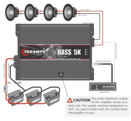
Examples of connections in the power supply input. Note: Required battery bank capacity: At least 210Ah
