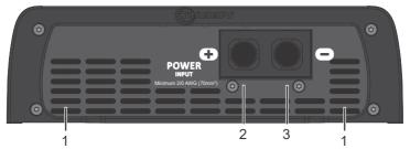
**1 - FANS:** This amplifier has two internal ventilation fans. For perfect functioning, the amplifier must be installed in a cool and aired place with at least 1" (25mm) space around the heatsink for proper heat spreading. The usually working temperature of amplifier is 65°C.
