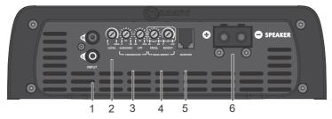
**1 - INPUT (R and L):** Inputs of signals to be amplified. Connect these signals to RCA outputs of Head Unit, using good quality shielded cables to avoid noise influence.
