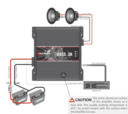
Examples of connections in the power supply input. Note: Required battery bank capacity: At least 115Ah
